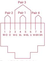
Figure 4: Eight-Position jack pin/ pair assignment (T568B)
