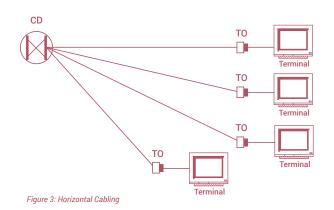
Horizontal cabling at Institutions shall consist of a minimum Enhance Category 6 from a local wiring closet to the room sockets. These cables are presented at both ends with RJ-45 type sockets. Telephone circuits shall also be delivered over the Category-6 cable as a minimum cable with a convertor plugged in at the client end to allow the connection of a normal telephone plug.
